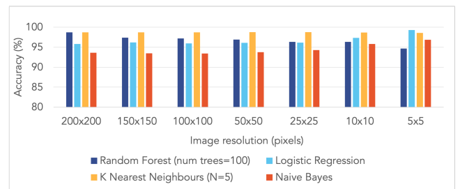
Figure 6: Leave-one-out cross-validation accuracy for the gating classifier at different image resolutions across all participants for different classifier types.
