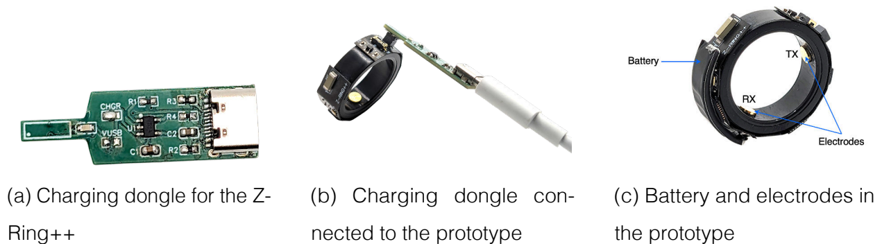
Figure 6.25: Components of the Z-Ring++ system
